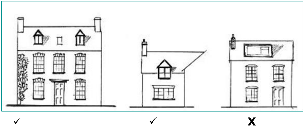
Fig. E20 – good and poor examples of dormer windows.
